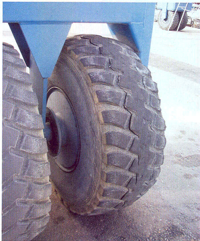
Left: The Marine Travelift pinned-type sling that failed. Right: Cracks in the lift's right tire indicate poor maintenance.
