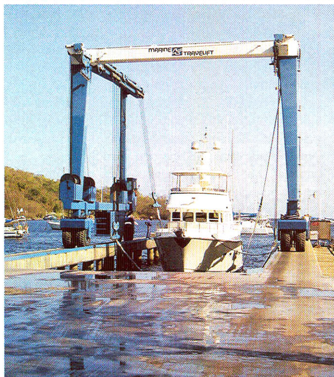
Top: Our Nordhavn before the accident. Middle: Peake Yacht Services' 150-ton Marine Travelift. Above: Centered in the lift and lines secured around her, our boat is ready for haulout.
