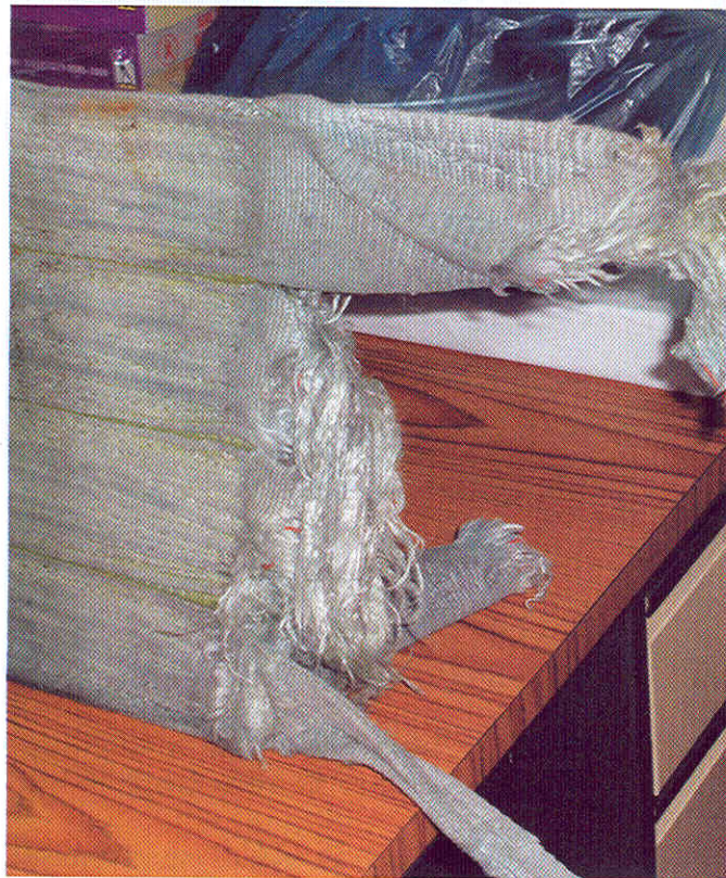
Left: The Marine Travelift pinned-type sling that failed. Right: Cracks in the lift's right tire indicate poor maintenance.
