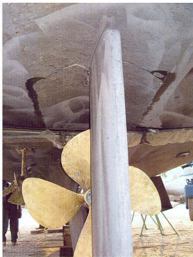
When the rudder shoe hit the concrete, the force pushed the rudder straight through the hull.
